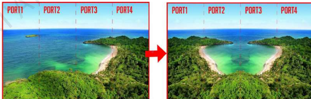
Figure 6-15 Left-right mirroring of images loaded by Ethernet ports 1–2
