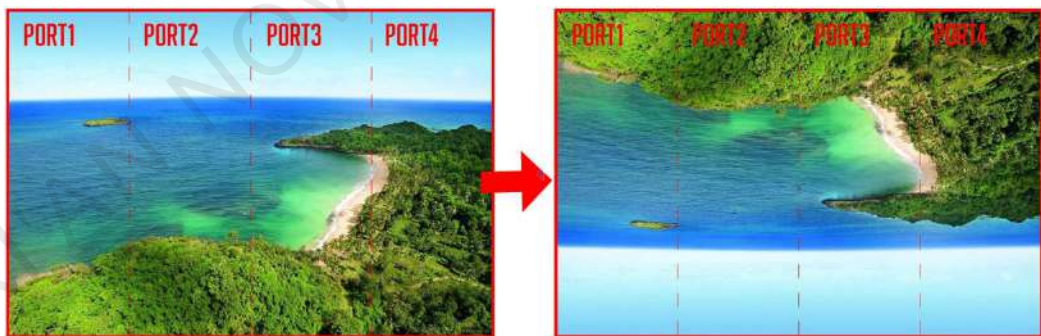
Figure 6-18 Top-bottom mirroring of the entire image
