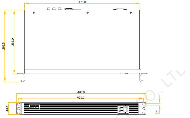
Tolerance: ±0.3 Unit: mm
